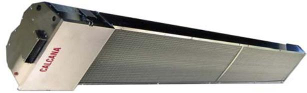
*Calcana heaters are available in 40,000 to 75,000 BTU's, have patent-pending variable heat settings, and come in 5, 10, 15 or 20-foot lengths which can be combined to achieve any length of configuration required.*
